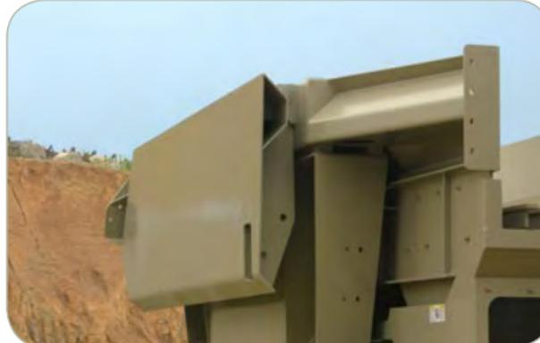
Heavy duty, folding wing, hopper extensions increase live storage to 18yd<sup>3</sup> capacity. Width at rear is 14'-11" capable of accepting loader feed from the rear of the plant.
