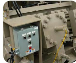
A position sensor automatically re-sets the crusher after relief.
