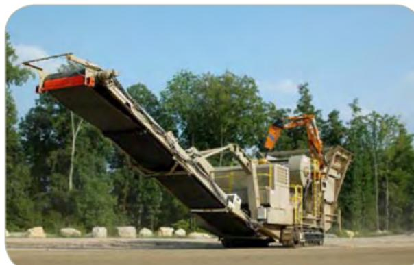
A 10 ft., manual fold, conveyor extension increases discharge height of the conveyor to 12'-10" (underside of belt scraper).
