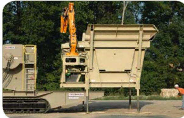
Hydraulic lift kit for the feeder module. Includes 4-point hydraulic lift package with 8 Hp gas engine.
