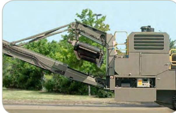
Adjustable height, self-cleaning permanent magnet discharges to the side of the plant.
