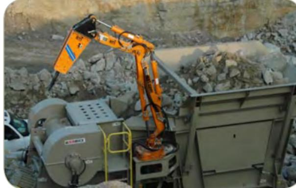
Hydraulic hammer (BTI MBS10-425X) 1,100 ft-lb class breaker with 10' boom includes handheld wireless remote control.
