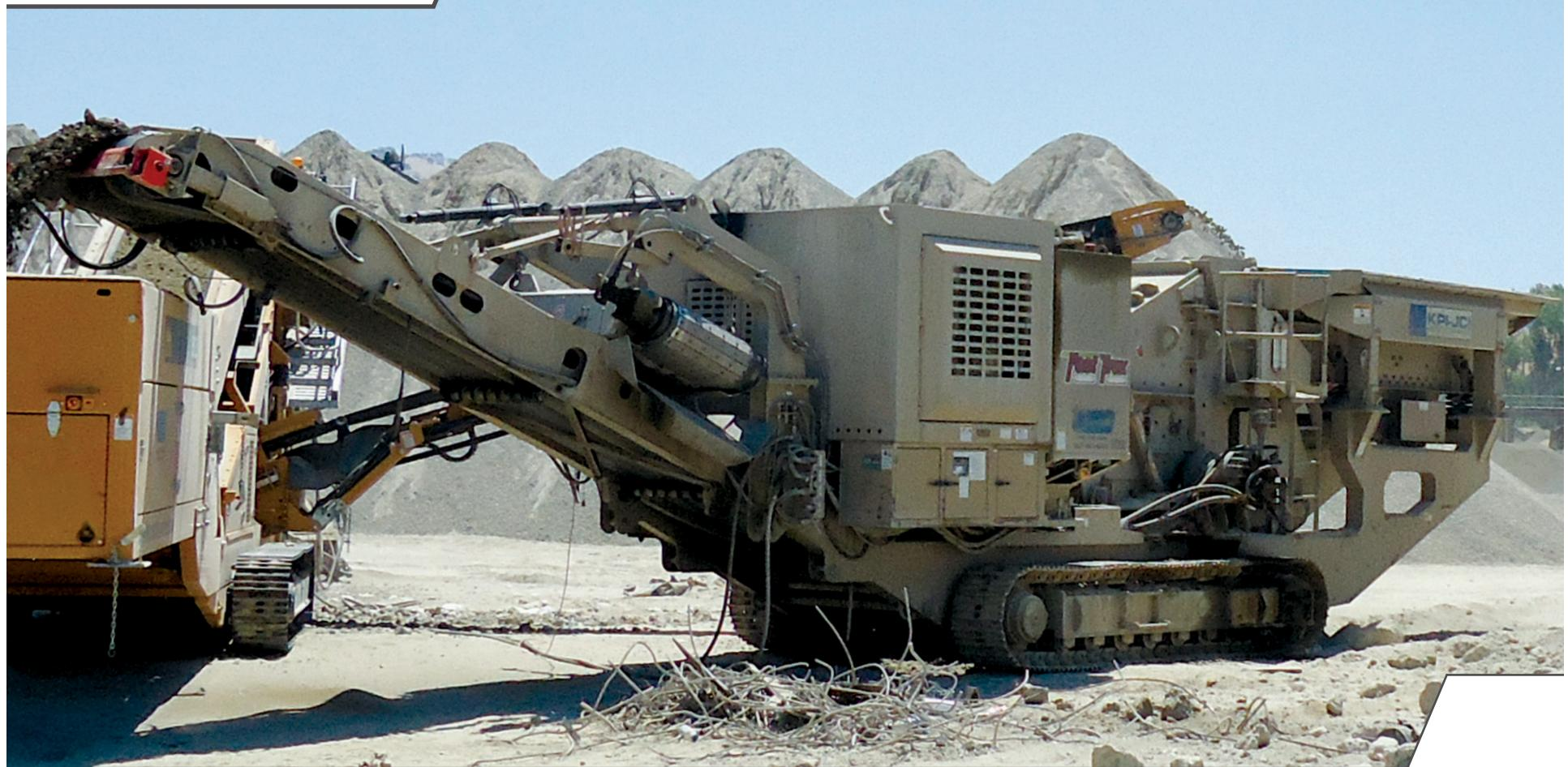
The Fast Trax® FT4250 is a mobile crushing plant that features an Andreas Impact Crusher for processing aggregates and recycled materials with a capacity of up to 500 TPH. As with all FT mobile plants, the FT4250 plant provides easy-to-reach engine controls, quick setup and easy-to-access grease points for routine service. The FT4250 provides simple to use hydraulic plant controls and crusher adjustments.
