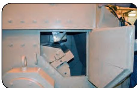
Inspection doors are located on both sides of the PA6060, allowing quick and easy access.
