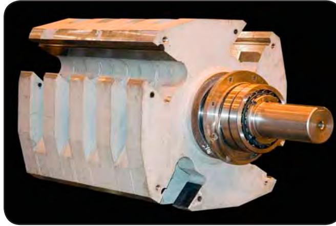
A massive solid type sculptured rotor delivers both high inertia for optimum crushing performance and solid backing support for the blow bars. This results in longevity and lower costs, even in rugged primary crushing.
